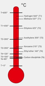
Figure 1: Temperature classes [°C] of equipment group II, according to European standards and ignition temperatures of relevant substances.
