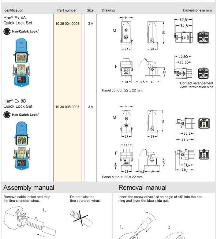
Push the fine stranded wires into the Han-Quick Lock® contact and push the blue slide with a screw driver<sup>1)</sup> until it comes to a stop.
