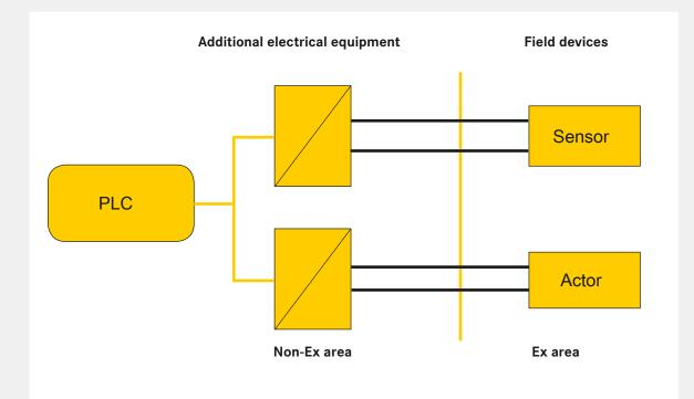
Figure 7: Han<sup>®</sup> Ex is a comprehensive connector system allowing for the safe transmission of power, signal and data between Non-Ex and Ex areas.
