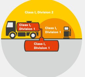
Figure 2: Classes and divisions using the example of a gas station acc. to NEC 505
